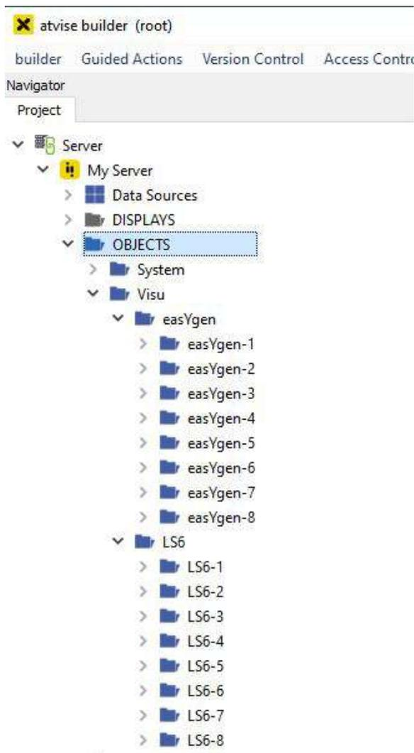
The used Modbus protocol for receiving easYgen data is 5016 and for LS6 data 5300. The nodes in the easYgen 1-4 folders are activated by default because they are used in the default visualization. All other data folder (easYgen 5-8 and LS6 1-8) are disabled by default. Refer to the easYview manual on how to enable additional device connections.
