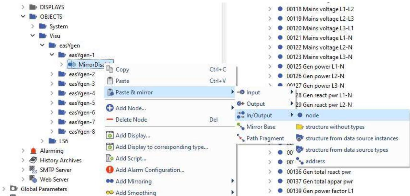
Enter a name for the new datapoint. In this example, we take the same name from the Modbus list and add the extension "- raw" because it is the raw Modbus value without formatting.
