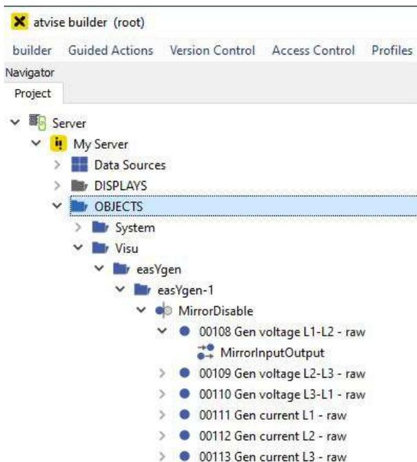
Data points with the extension “- raw” are the main data points which have exact the value like transmitted from the easYgen-3000XT. These data point may needs to be formatted to match the easYgen data before transmitted via Modbus. To show the data formatted, use the parameter “value\_postdecimalposition” and “value\_forcedecimalfractionposition”. For details about the data format, refer to the easYgen manual→Protocol 5016.
