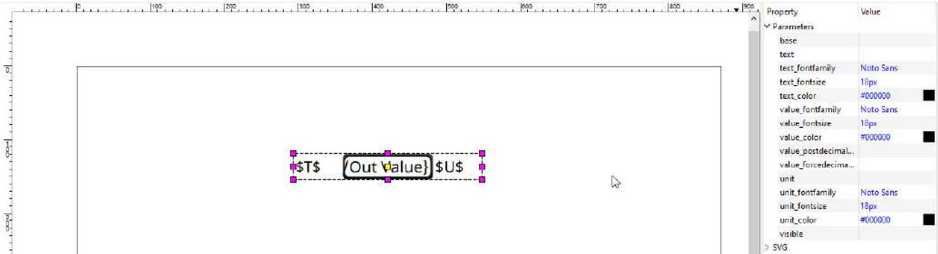
Enter the needed attributes for “base”, “text” and “unit”. To enter the “base” (reference to the datapoint) click on the three dots to select a datapoint from a list.
