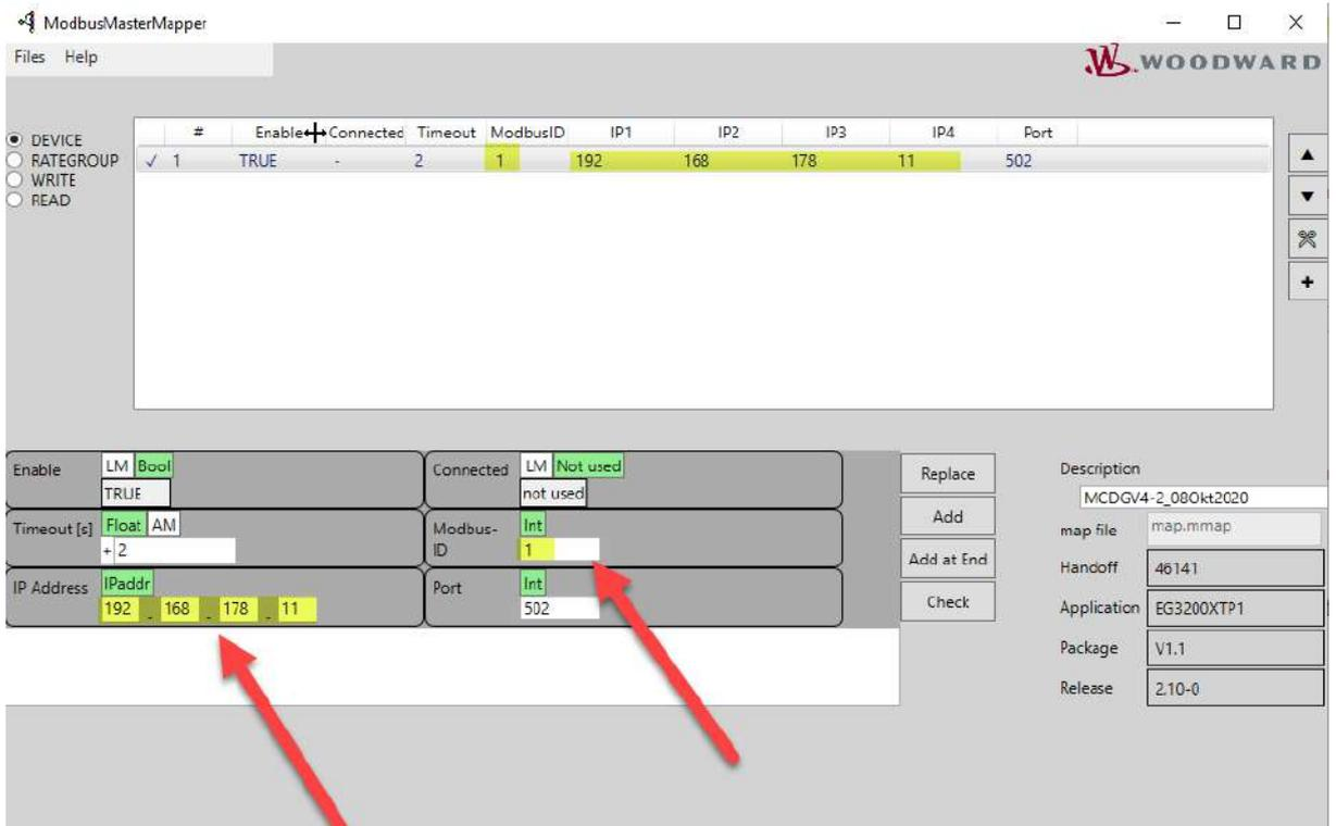
The “Device” menu defines external devices, to which the easYgen-XT as Modbus Master will connect.
