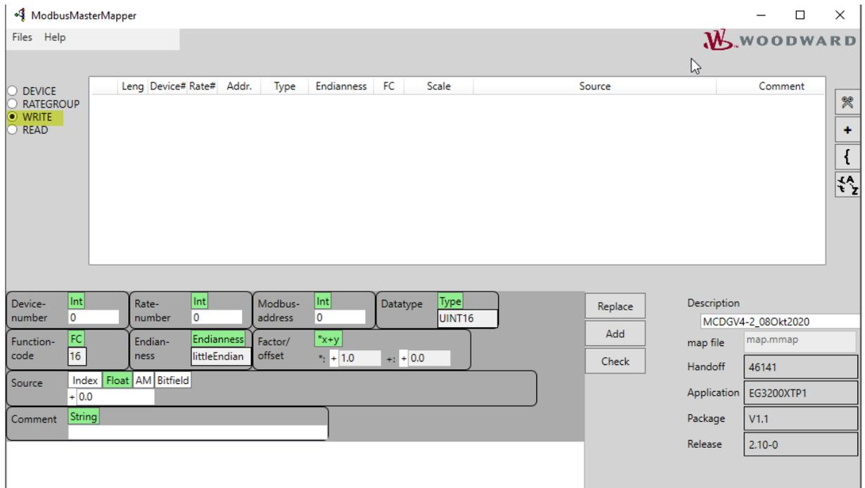
The “Write” menu defines a Modbus command to be transmitted. The easYgen-XT periodically sends a Modbus-command 16 “write multiple” to transfer data to the MCDGV4.
