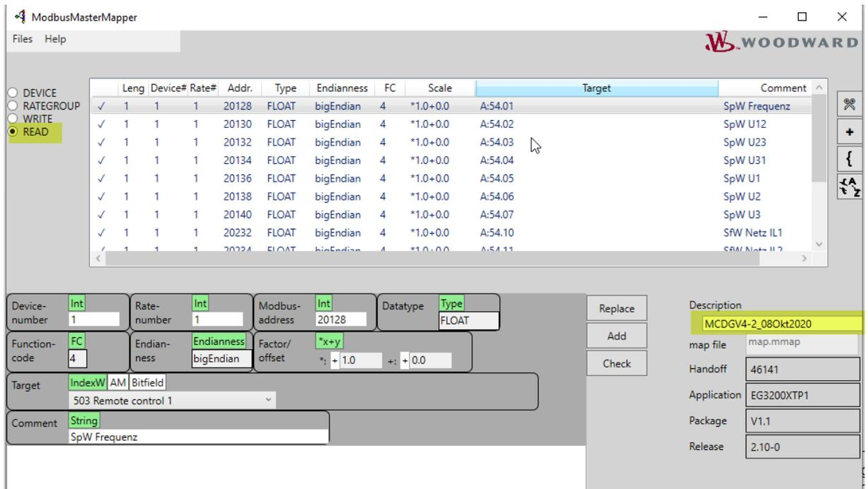
The “Read” menu allows for defining a Modbus read command.
